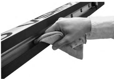
When resistance seems to have increased or movement begins to feel "sticky", wipe all upper and lower inner surfaces with paint thinner to remove dry gummy lubricant build up.
