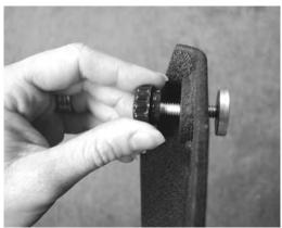
Rotate leveling knob up or down until blase plate lays flat on the surface on which it is placed.
