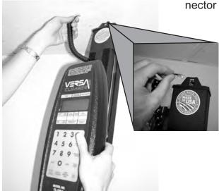
Place the display console (Module) on the machine in contact with the velcro strips.
